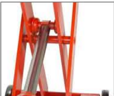
Safety distance between scissors.
