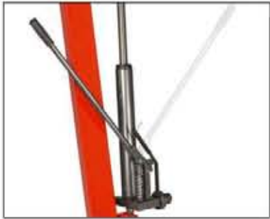
Swivel hydraulic unit. The pump piston spring improves operation.
