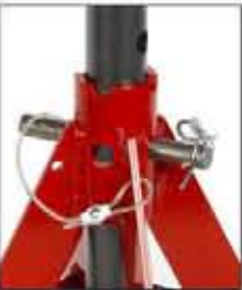
Pin secured to the stand to avoid loss.
