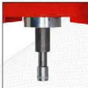
Manual screw extension for quick approach and fine adjustment.
